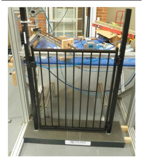
As per 'AS1926.1 Set 2012- Swimming Pool Safety Standards Set- Section 3.6- Durability of a Gate Unit' only.
