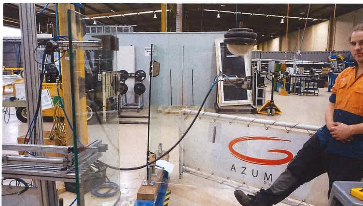
Figure 3: 25 kg Gate Open
